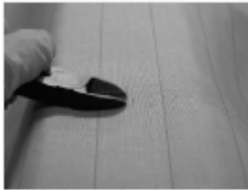
Fig. 5.3.4-1: Shortening pins with a diagonal cutter
