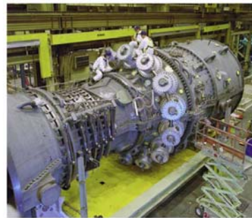
Fig 15. GE-9H gas turbine is prepared for testing (Source: GE Power Systems)
